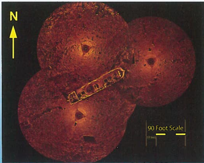
Sultan 360 Sonar 90 ft composite image. Brian Abbot, Nautilus Marine Group International, LLC
